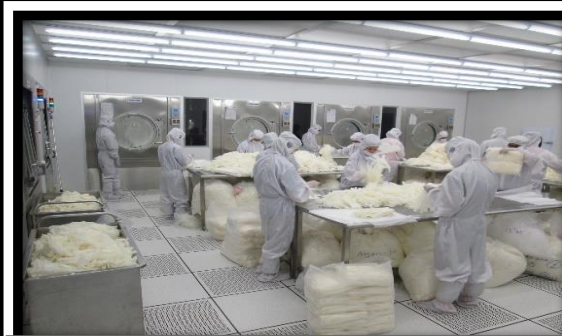
Class 100 cleanroom inspection
