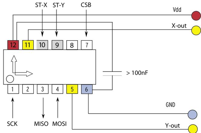
Self test can be activated applying logic "1" (positive supply voltage level) to ST pin (pin 9 and 10). If ST feature is not used pins 9 and 10 must be left floating or connected to GND.
