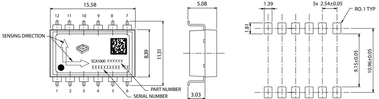
Acceleration in the direction of the arrow will increase the output voltage.
