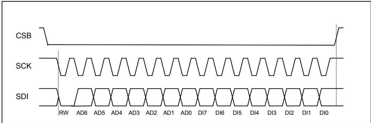
**Figure 10:** For three wire read protocol one extra clock between address byte and data out byte is required. Output data are changed on SDI (SDI=SDA) by SCK rising edge and should be latched by microprocessor during next SCK rising edge.
