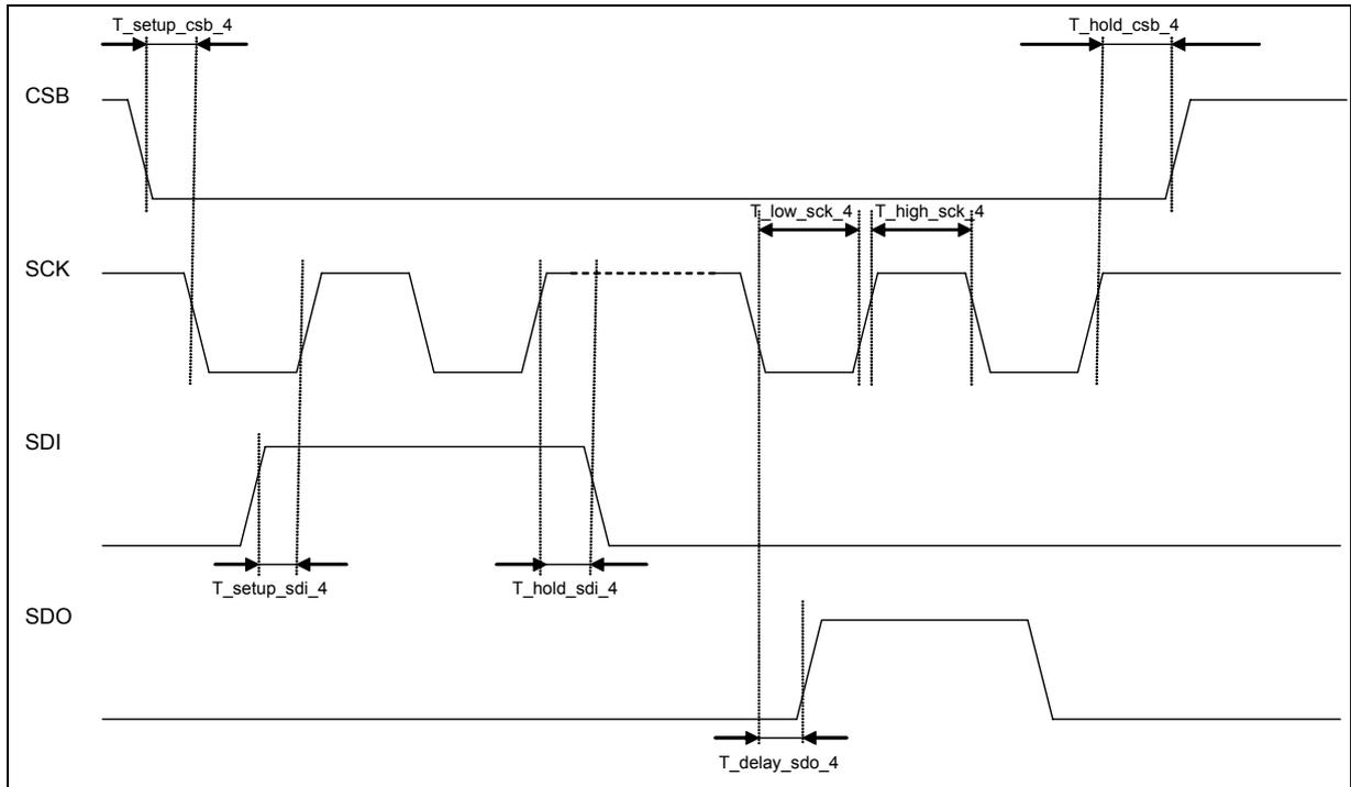
**Figure 5:** Four wire SPI bit transfer
