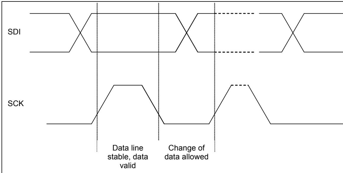
**Figure 14:** Timing diagram for I<sup>2</sup>C acknowledgement on SDI (SDI=SDA)
