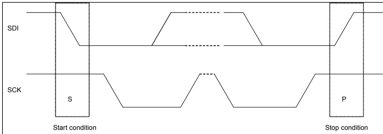
**Figure 13:** Timing diagram for one bit transfer with I<sup>2</sup>C interface (SDI=SDA)
